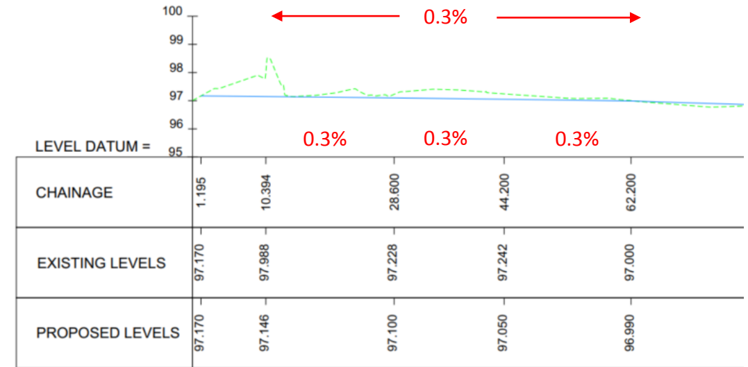
EASTERN CHANNEL – RIVER COCKER (LONG-SECTION)
